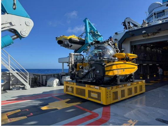
The submersibles are positioned on the working deck beneath the A-frame, which lifts and launches them over the stern of the ship. In contrast, the ROV Chimera is deployed via an L-frame system on the vessel's side.
