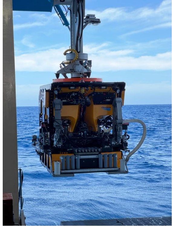
The submersibles are positioned on the working deck beneath the A-frame, which lifts and launches them over the stern of the ship. In contrast, the ROV Chimera is deployed via an L-frame system on the vessel's side.
