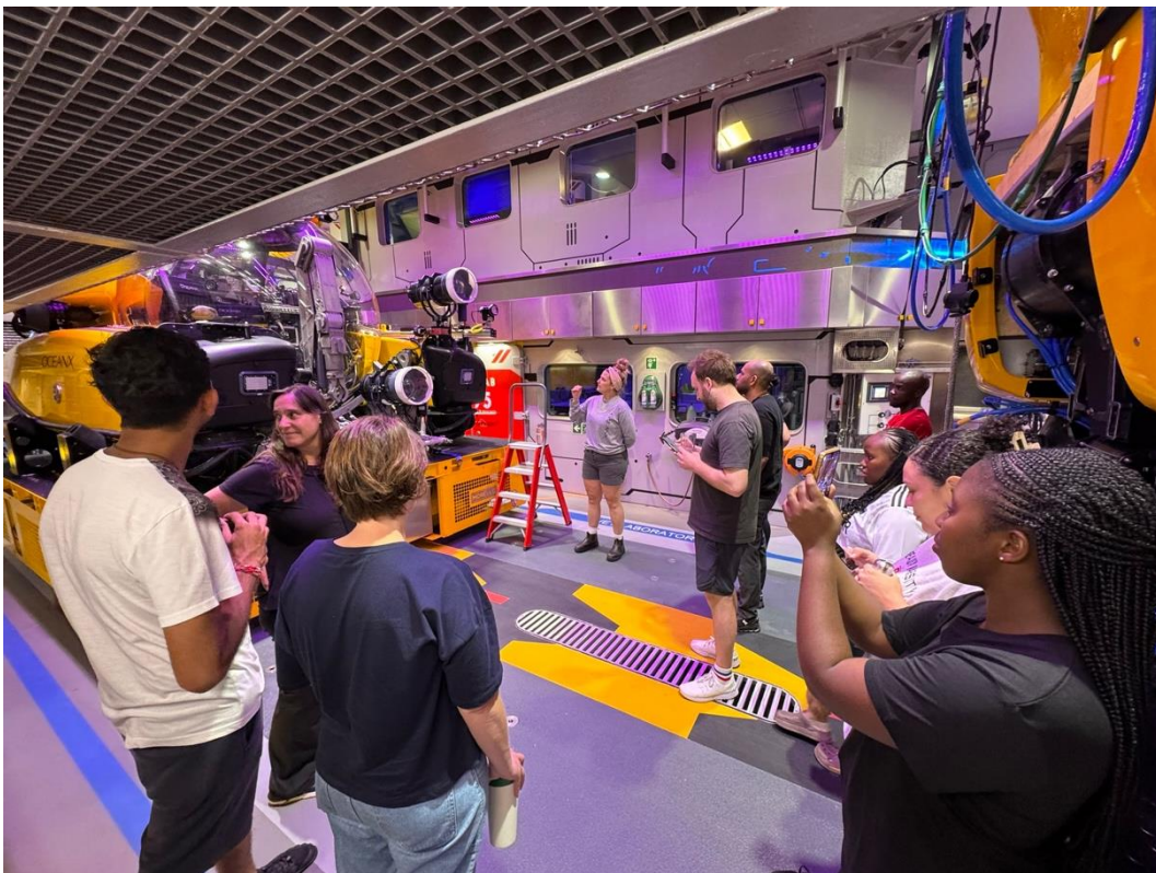
Everyone was deeply impressed when standing in the hangar and looking at the huge, 1000-meter-rated 3-person occupancy submersibles equipped with camera systems, manipulator arms, push corer, and sampling systems.
